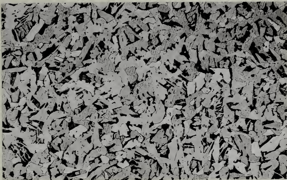
Figure 8. Microstructure of vane 4. 1% Nital etch. X 100
